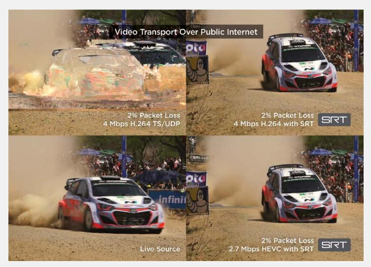
Figure 1: This image is divided into four quadrants to illustrate the impact of errors and error correction systems on video signals. The source video signal is shown in the lower left. The upper left quadrant shows the video degradation caused by a two percent packet loss rate. The two images on the right half of the illustration show how SRT can eliminate video impairments for two commonly used video codecs at two different bit rates.
